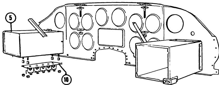
Figure 111. Gyro Fixed Instrument Panel Assembly (D2861 thru D4865)
