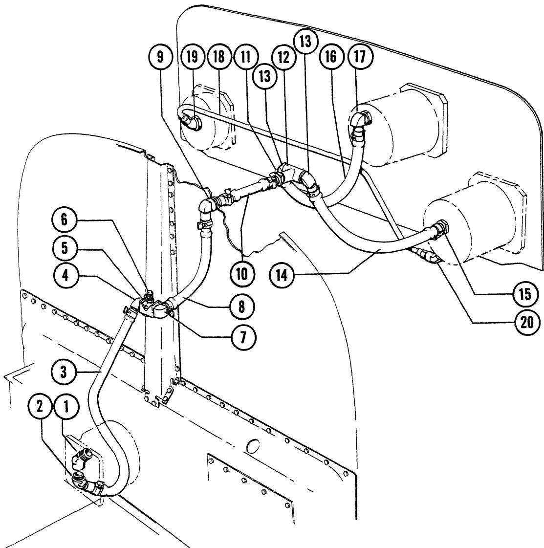
Figure 118. Gyro Instrument Plumbing System (D2681 thru D4865)
