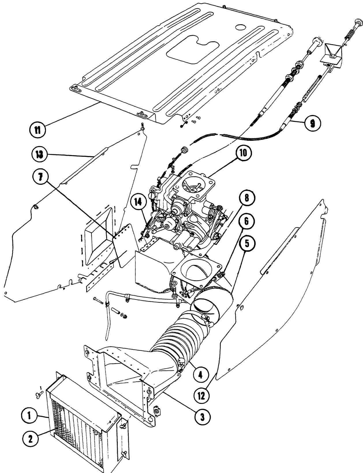
**Figure 82. Carburetor Induction System (D1 thru D1116)**
