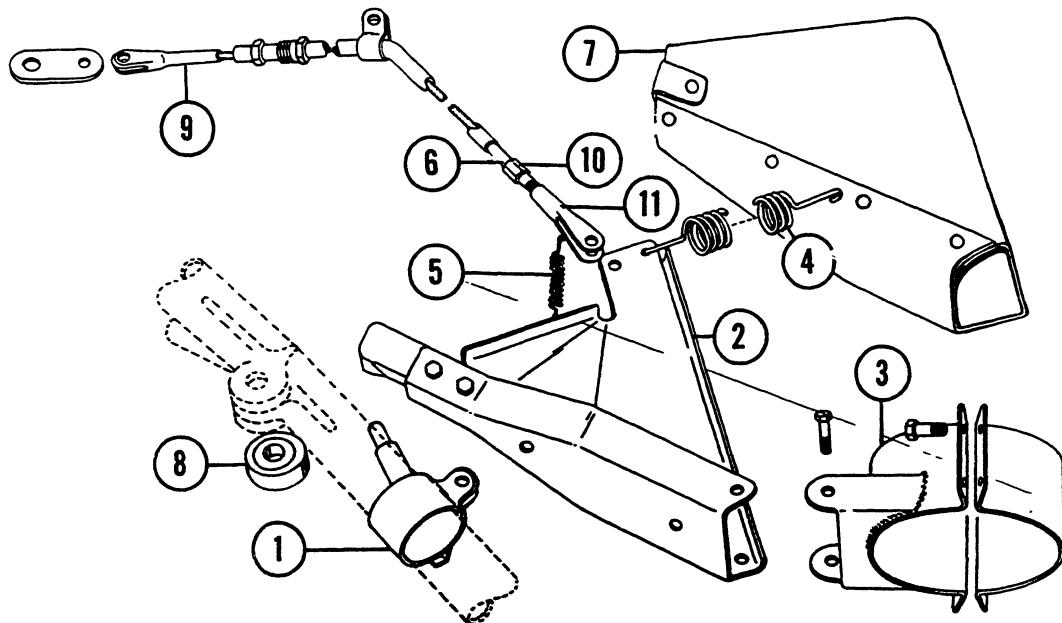
Figure 69. Main Landing Gear Up Lock
