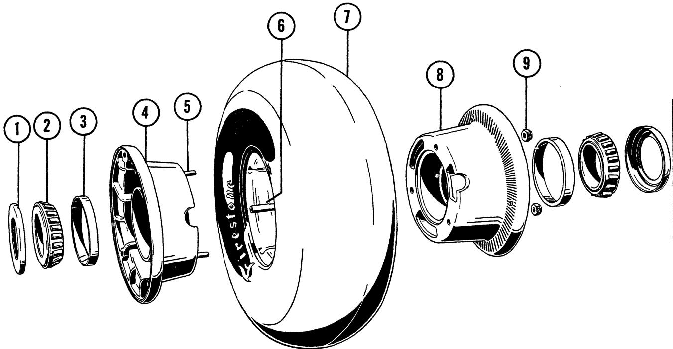
**Figure 53. Nose Wheel And Tire Assembly**
