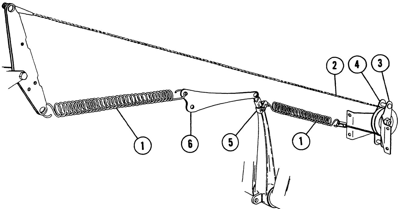
Figure 36. Trim Tab Bungee Mechanism
