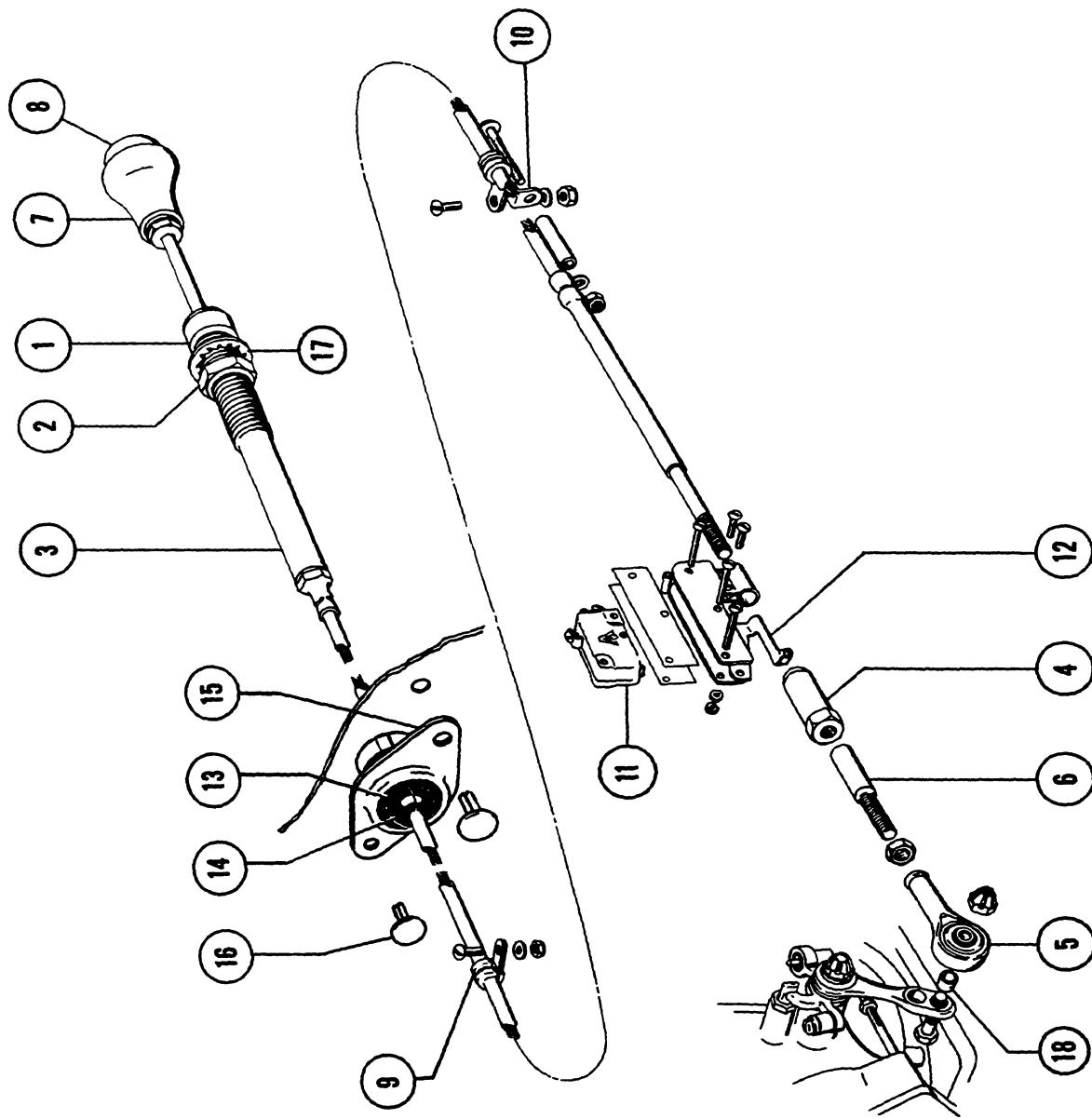
Figure 99. Throttle Control and Landing Gear Warning Switch
