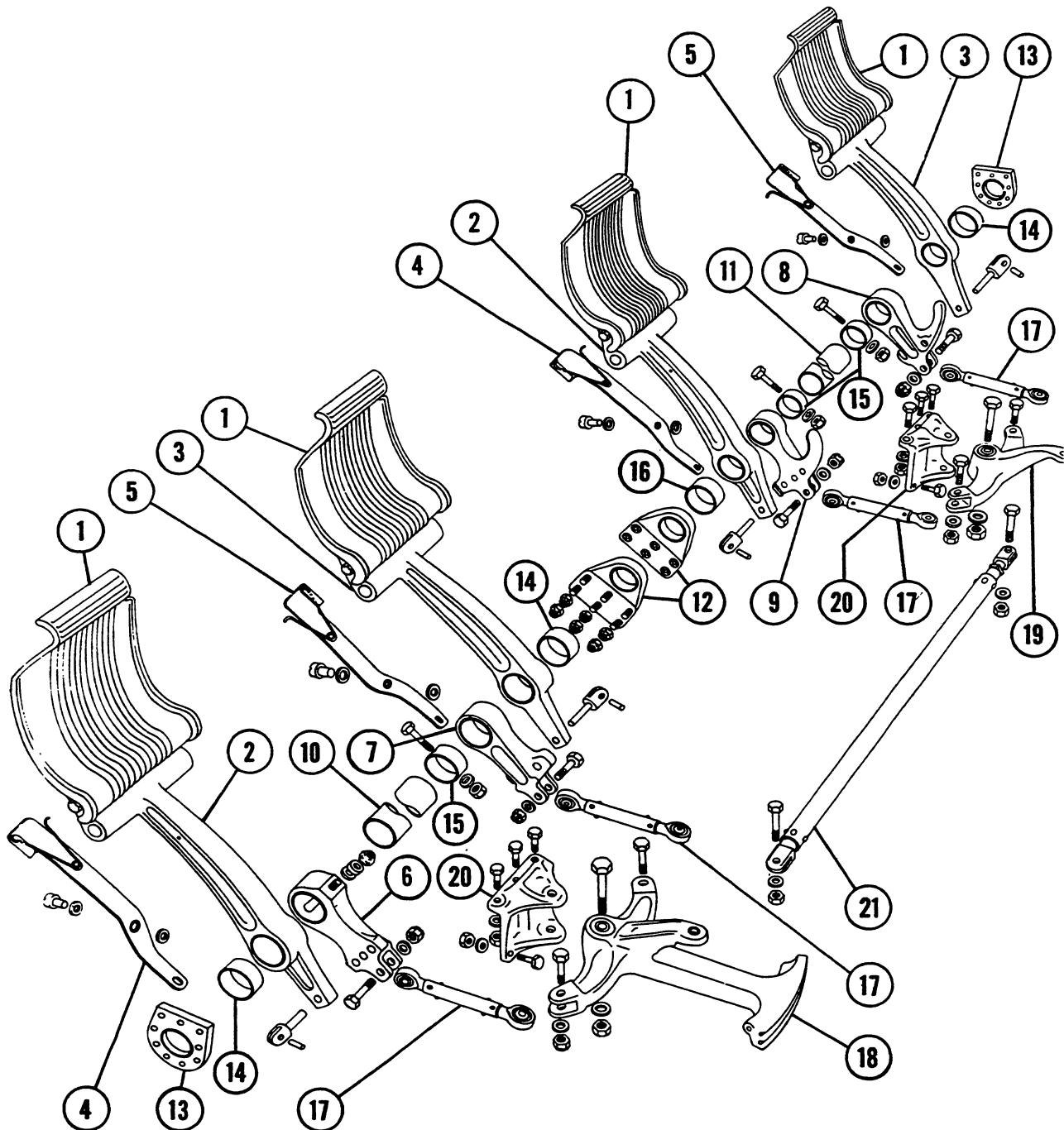
Figure 29. Rudder Pedal Assembly
