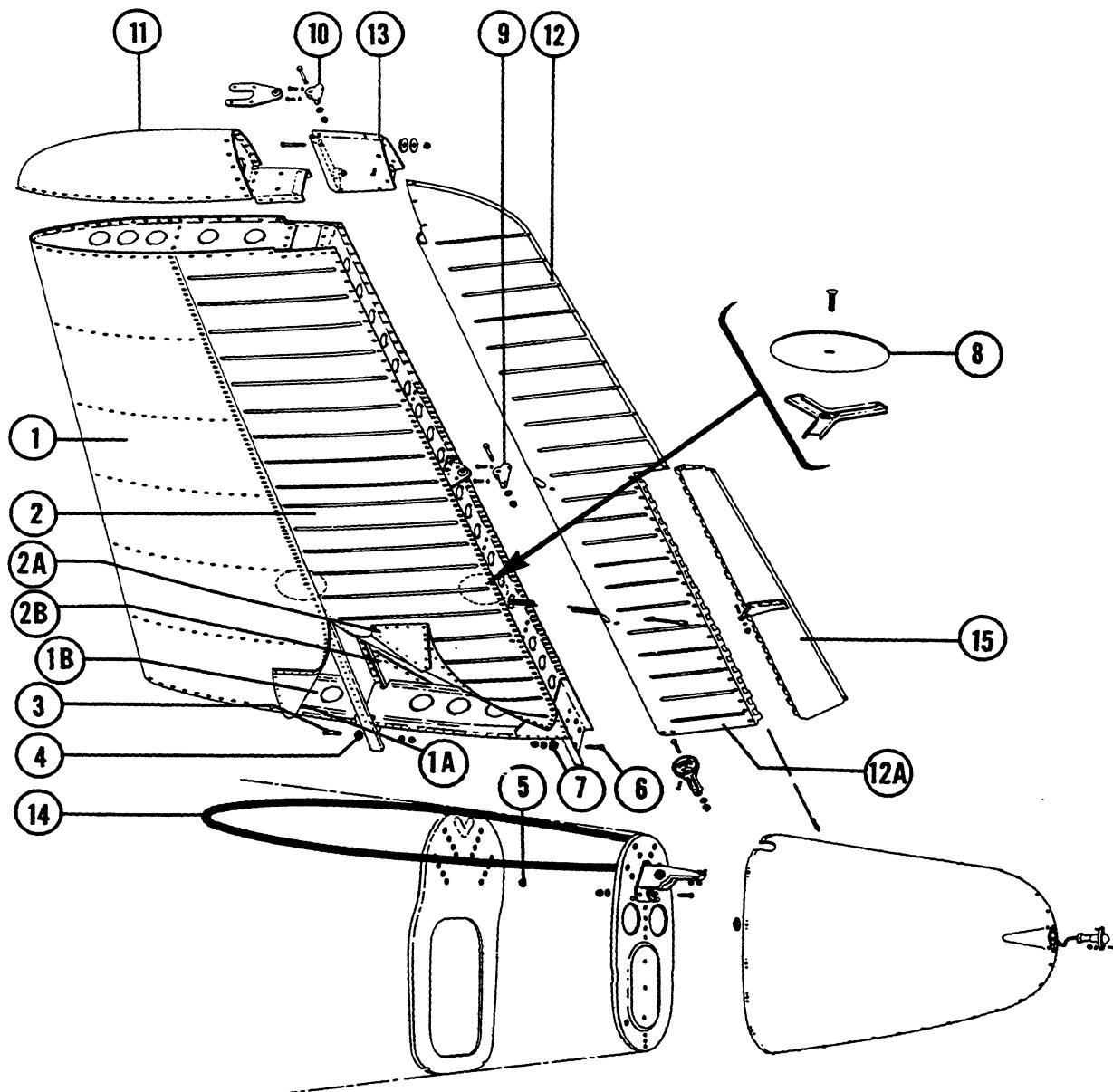
Figure 13. Empennage Group (D2681 thru D4865)
