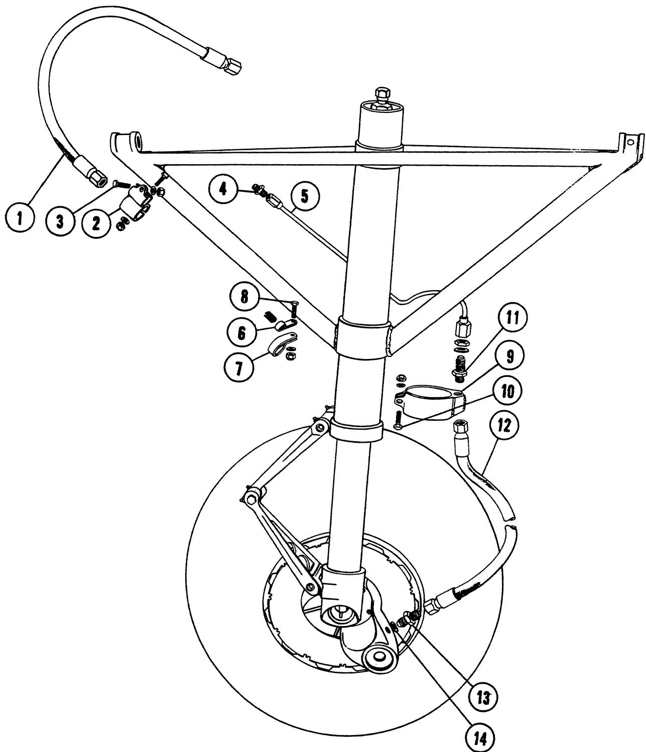
Figure 62. Strut Brake Piping
