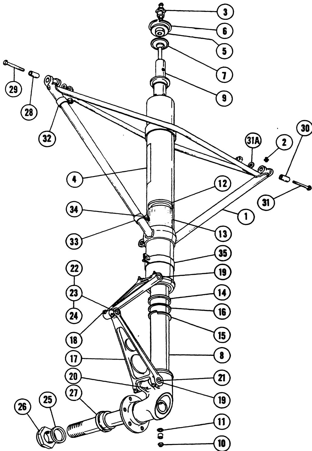
Figure 44. Landing Gear Shock Absorber Assembly (D2681 thru D4098)
