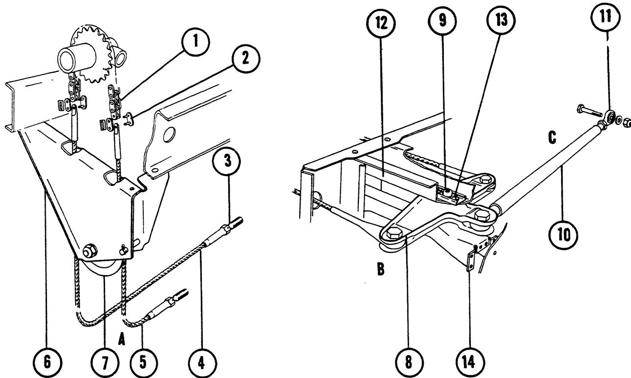
Figure 22. Aileron Control Sprocket And Bellcrank Assembly
