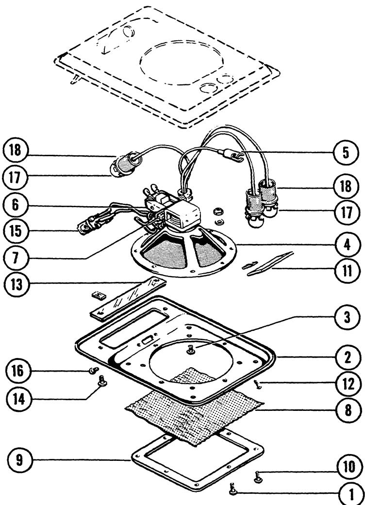
Figure 130. Dome Light and Radio Speaker (D2681 thru D4865)
