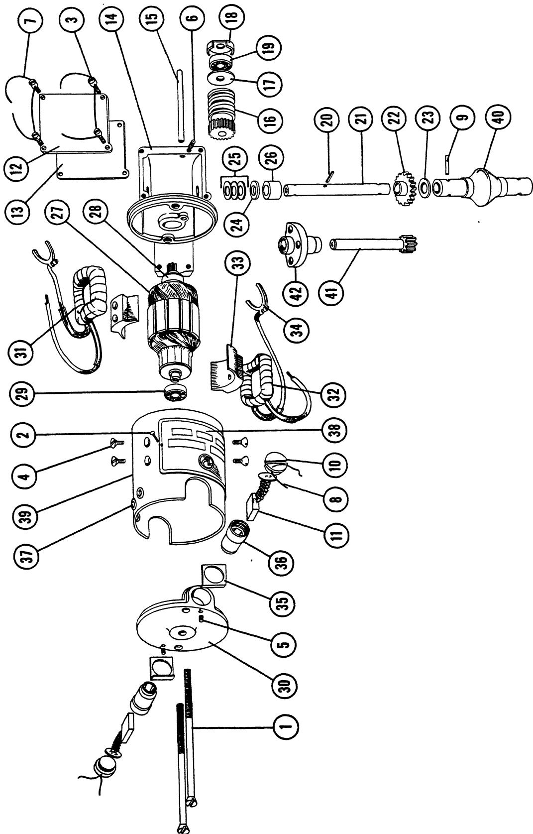
Figure 98. Propeller Pitch Motor Assembly
