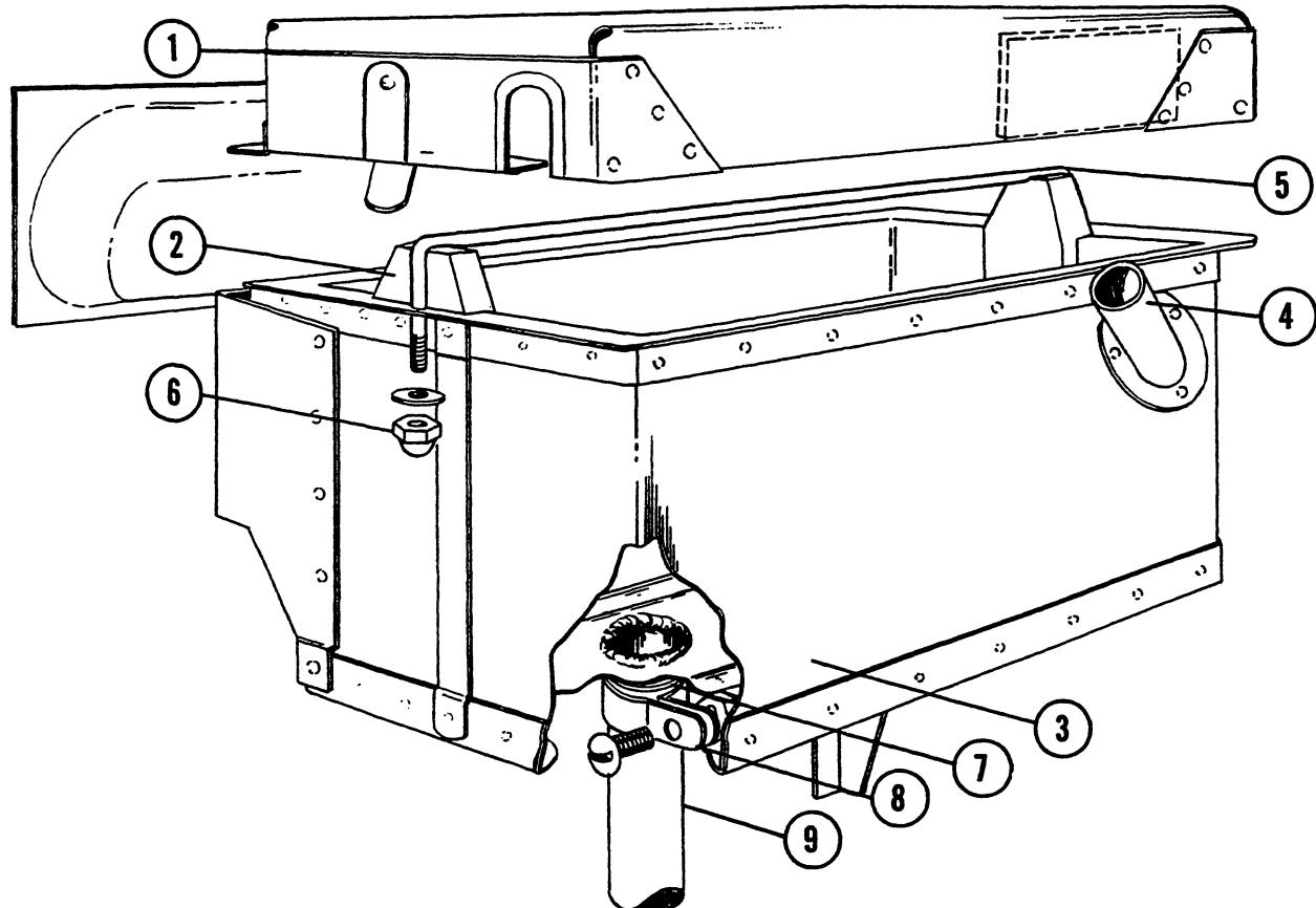
Figure 131. Battery Box Assembly (D1 thru D1116)
