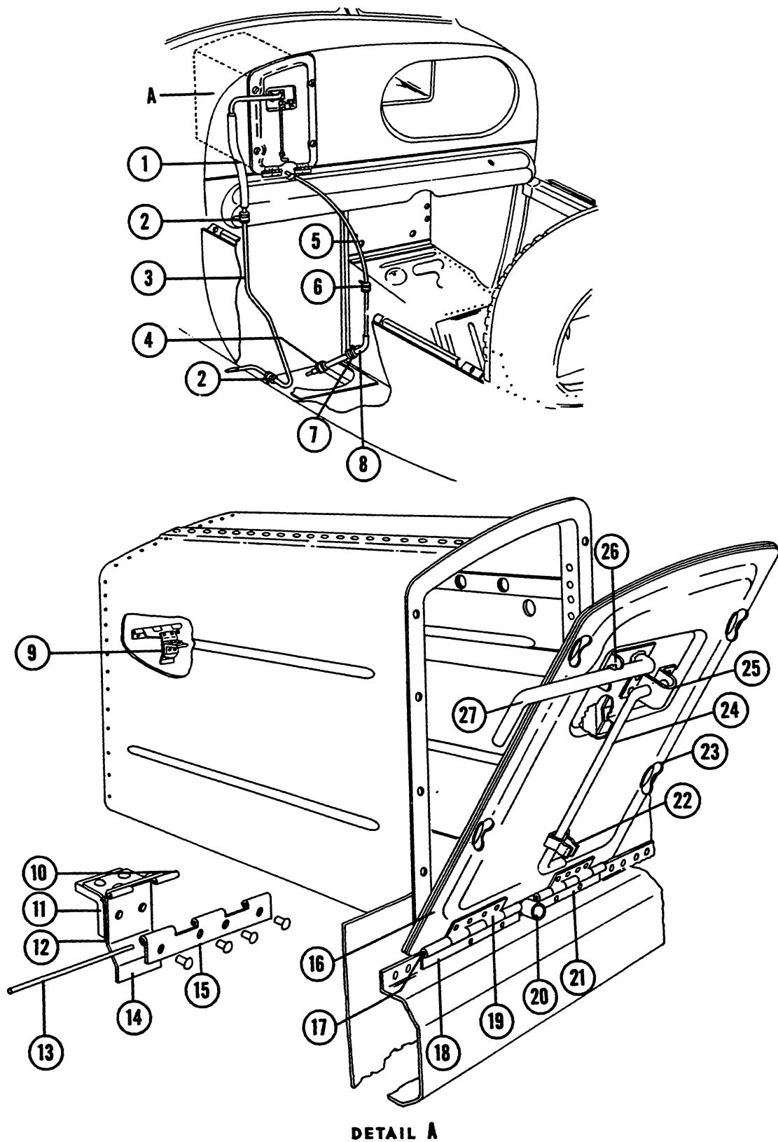
Figure 133. Battery Box Assembly (D1911 thru D4865)
