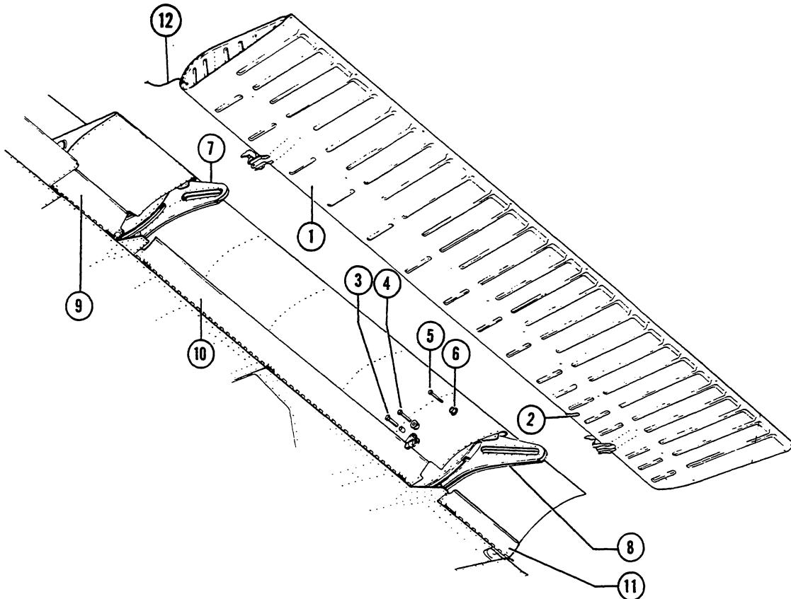
Figure 11. Flap, Flap Track and Flap Gap Doors
