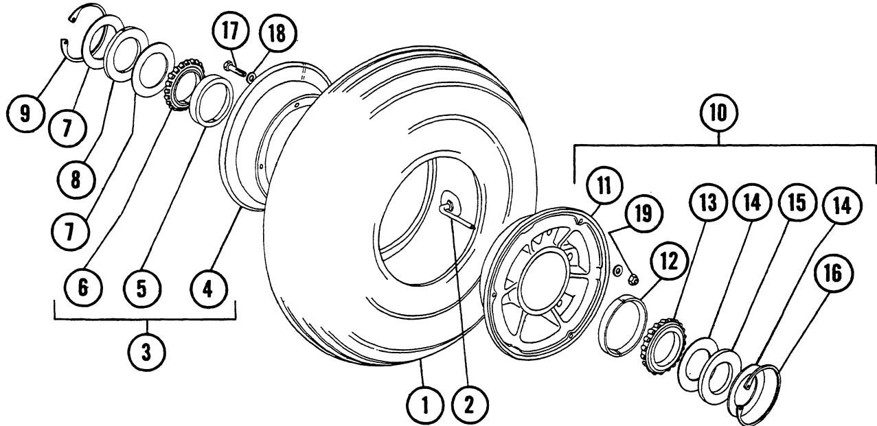
Figure 52. Nose Wheel And Tire Assembly
