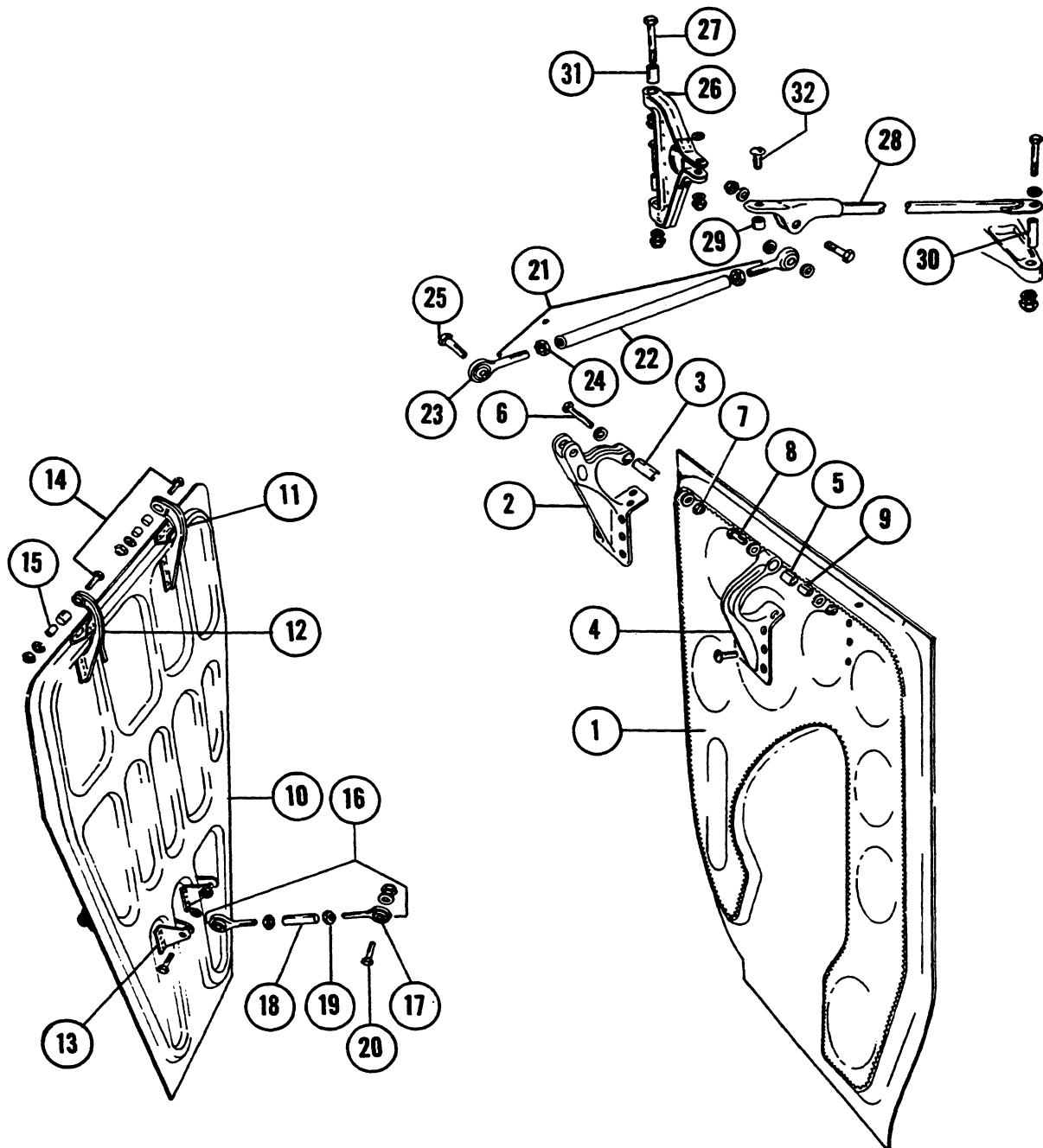
Figure 46. Main Landing Gear Door and Retract Mechanism
