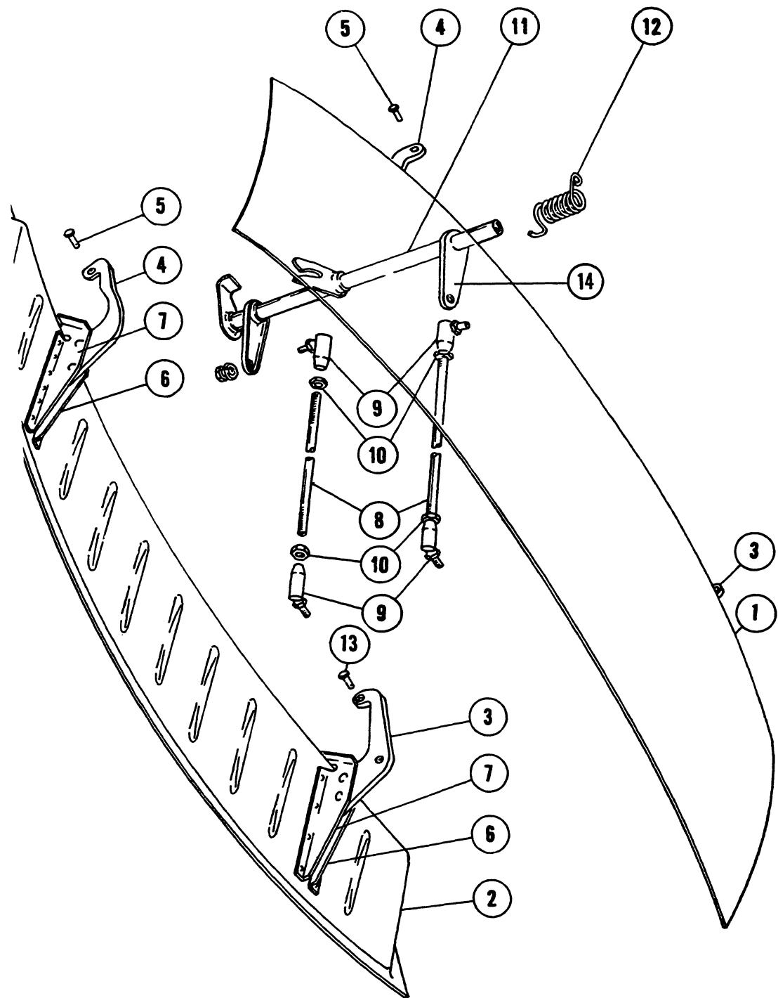
Figure 55. Nose Wheel Doors and Retract Mechanism
