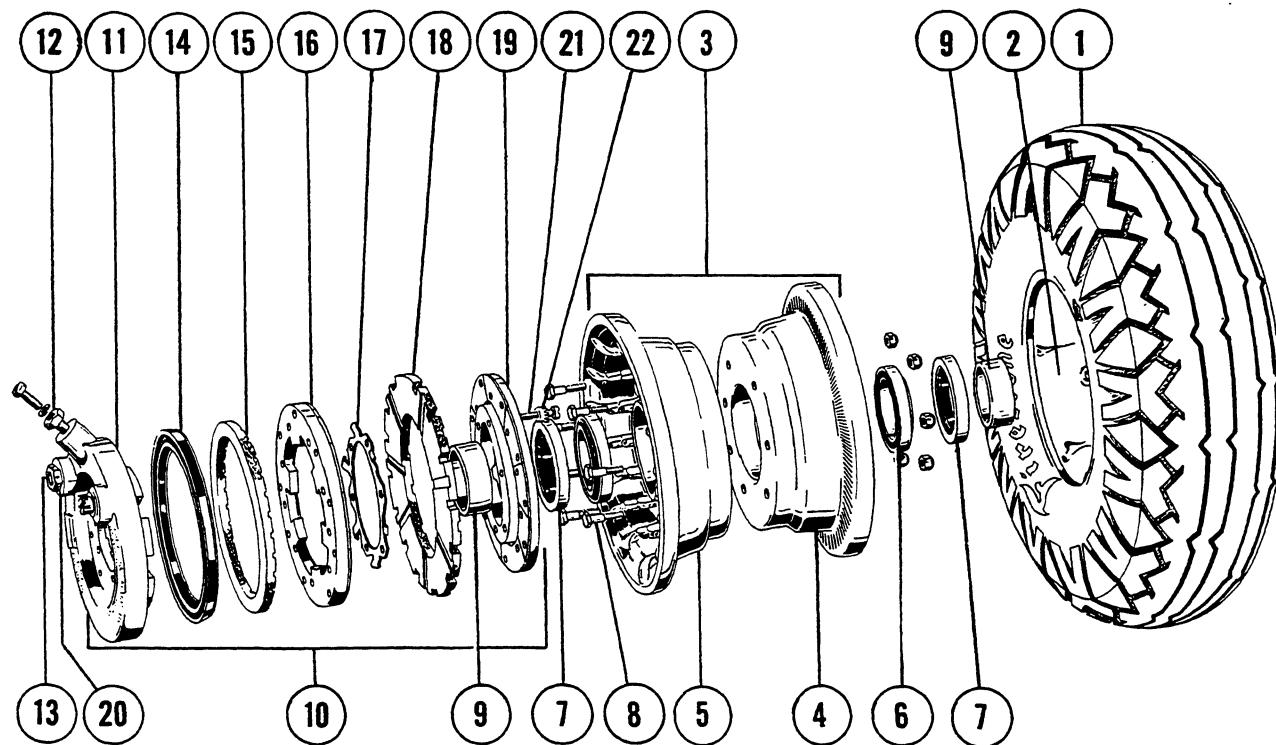
**Figure 48. Main Wheel, Tire, Tube And Brake Assembly**
