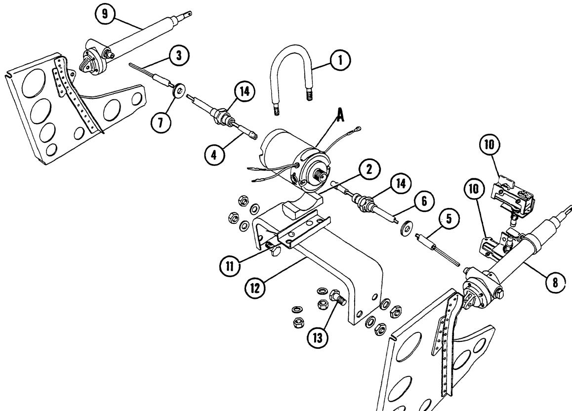
**Figure 14. Flap Control Mechanism (D1 thru D837)**
