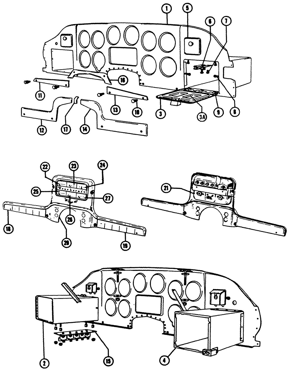
Figure 110. Fixed Instrument Panel Assembly
