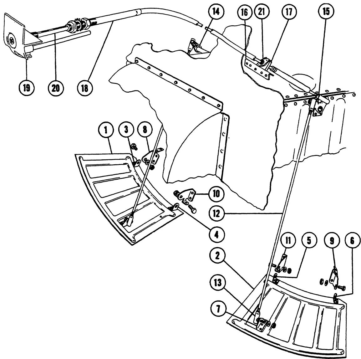
Figure 76. Cowl Flap and Control Assembly
