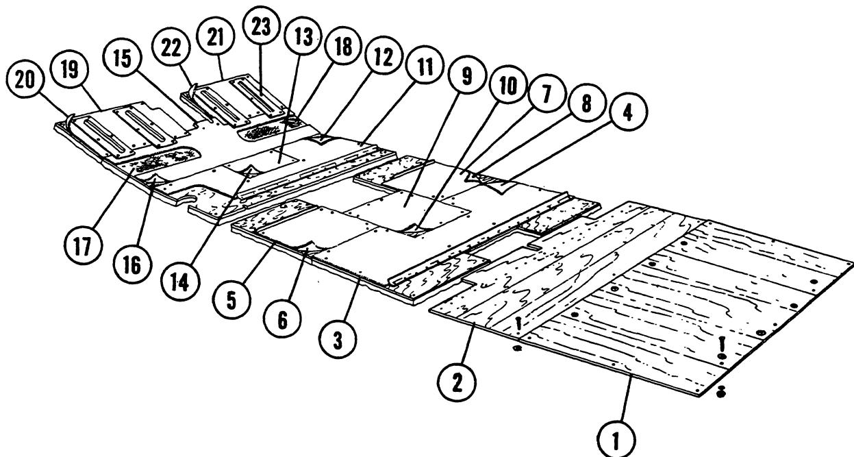
**Figure 104. Cabin And Baggage Compartment Floorboards**
