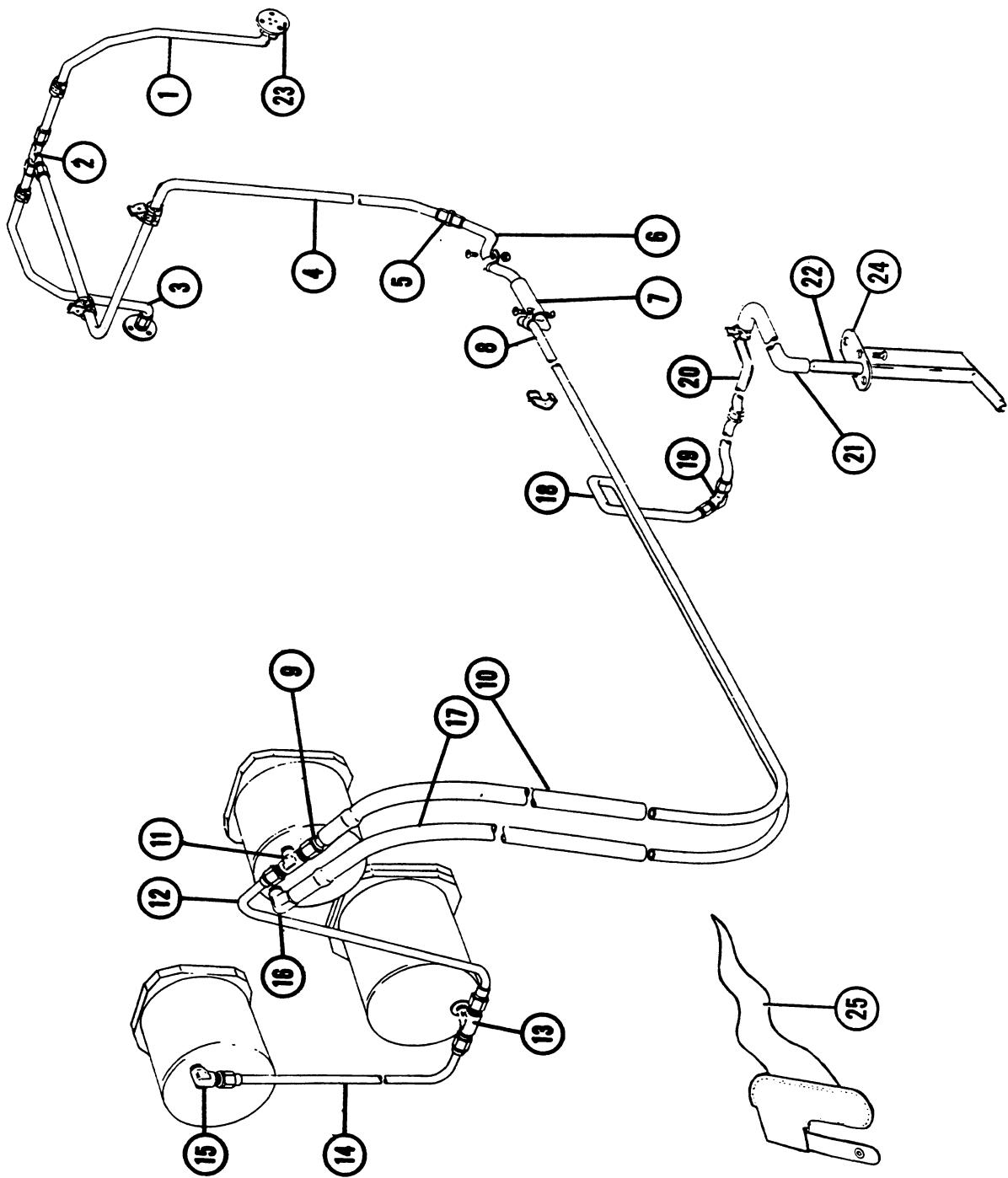
Figure 119. Static Pressure and Pitot Plumbing (D2681 thru D4865)
