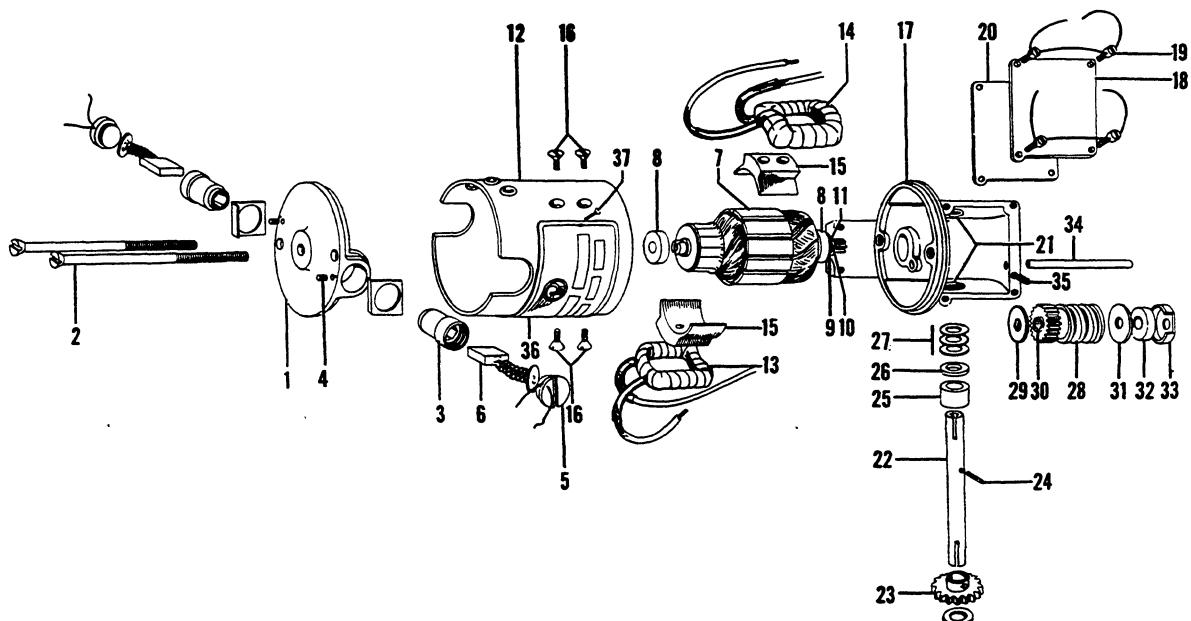
Figure 19. Flap Motor Assembly (D838 thru D4865)
