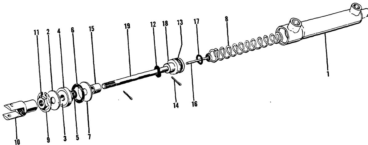
Figure 68. Brake Master Cylinder Assembly (Firestone Brakes)
