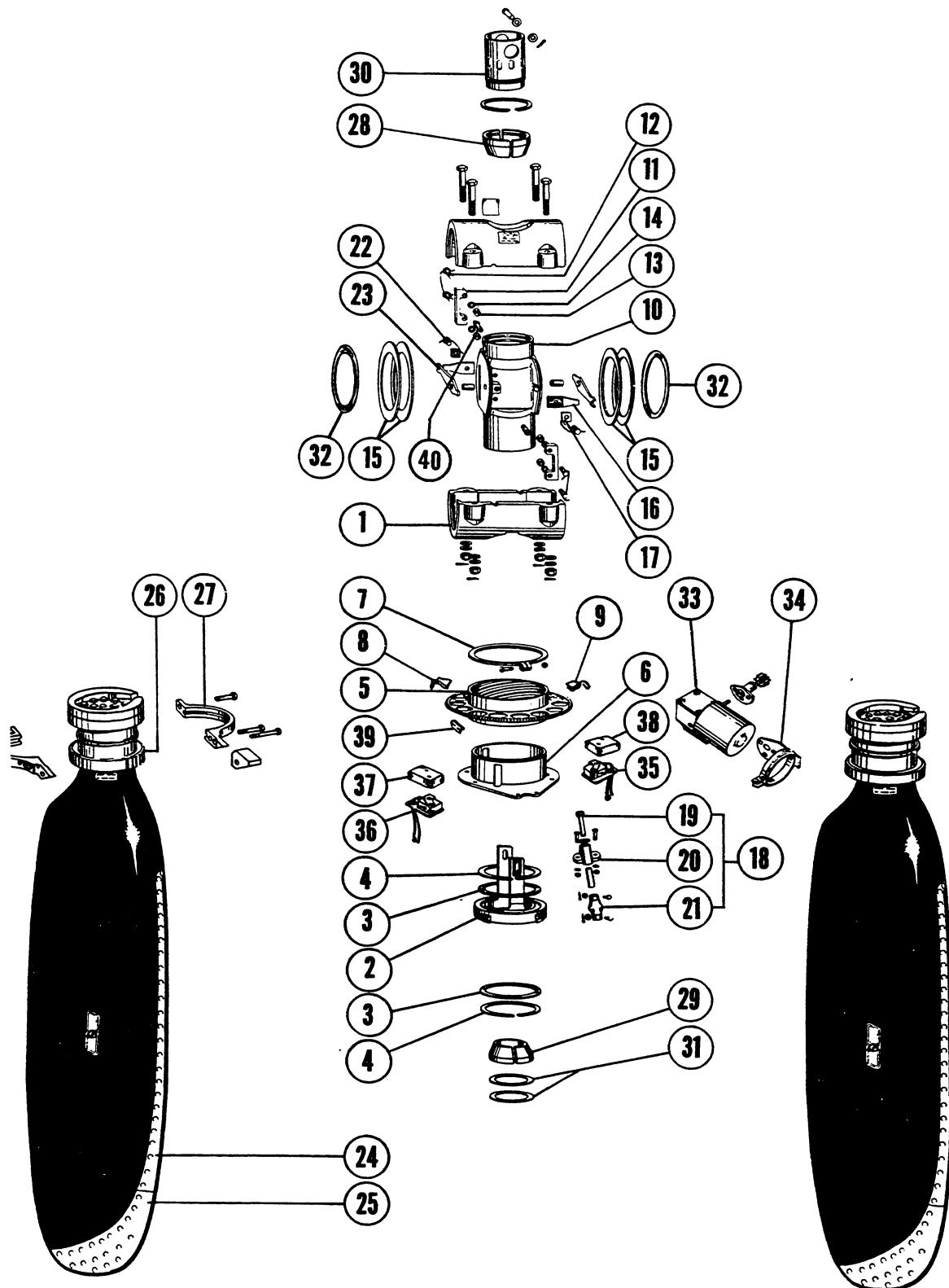
Figure 94. R200 Propeller Assembly
