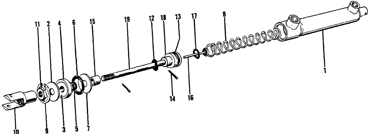
Figure 67. Brake Master Cylinder Assembly (Goodyear Brakes)
