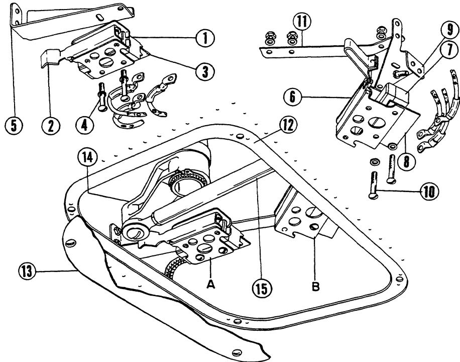
Figure 57. Landing Gear Switch Assembly (D1 thru D1500)
