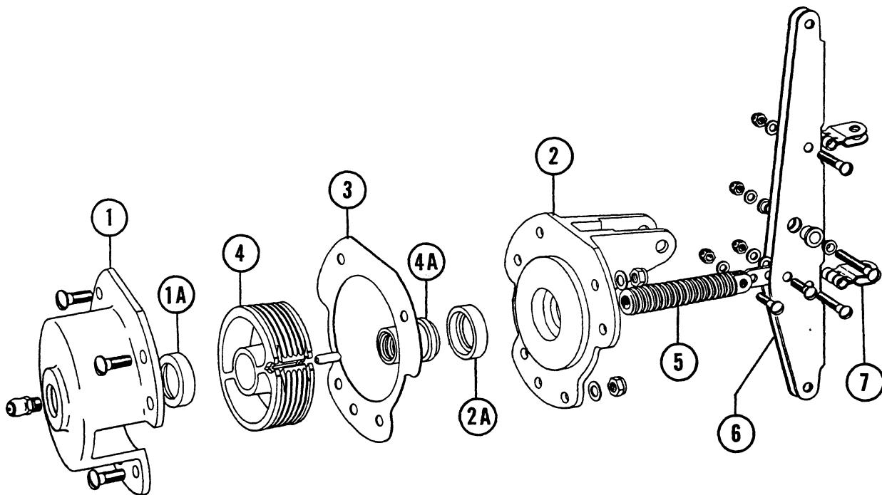
Figure 35. Trim Tab Actuating Mechanism
