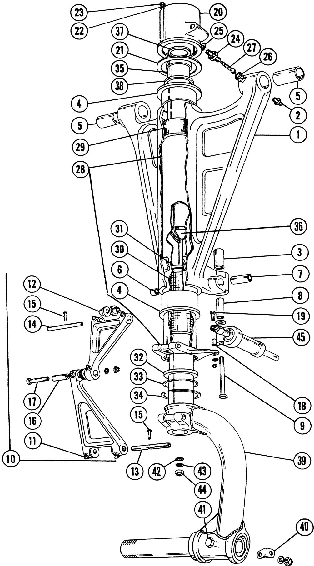
Figure 50. Nose Wheel Strut Assembly
