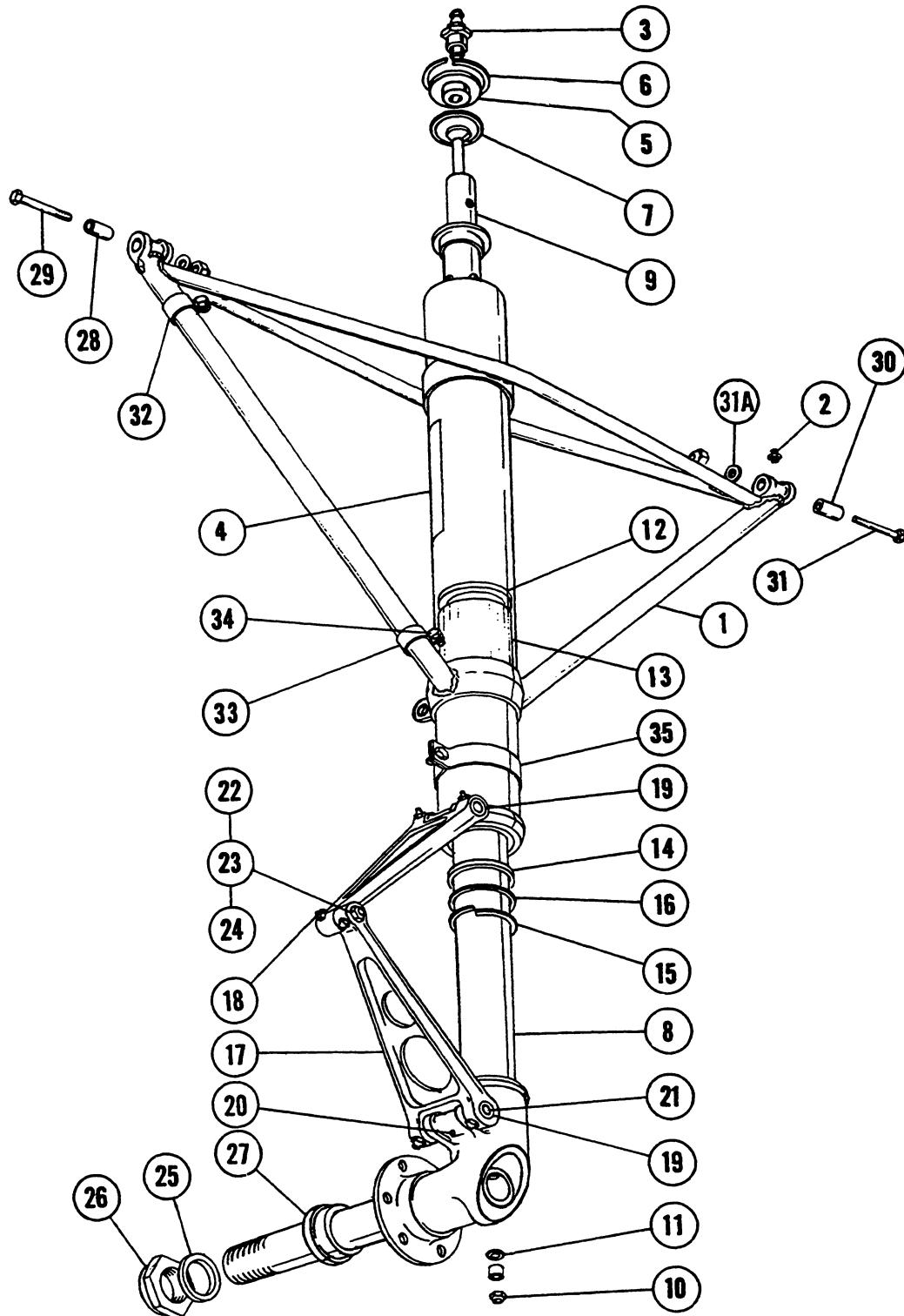
Figure 43. Landing Gear Shock Absorber Assembly (D1 thru D2680)
