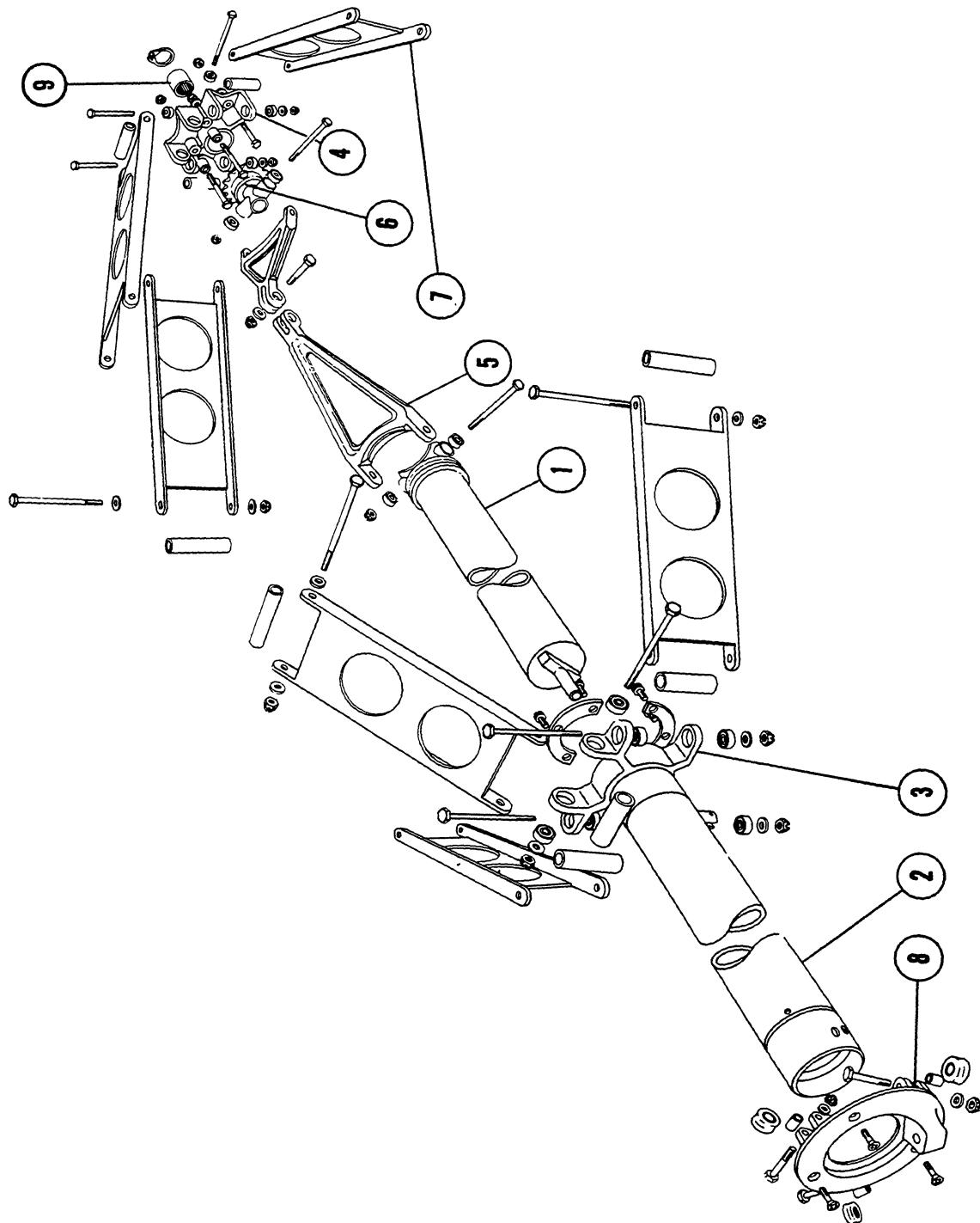
Figure 39. Control Column Assembly
