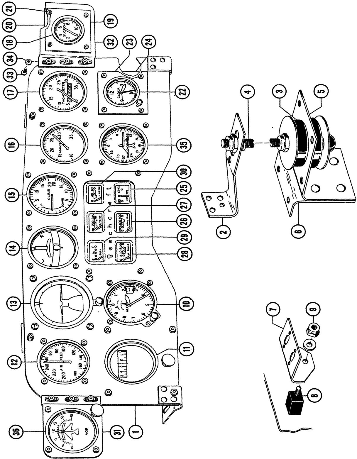
Figure 114. Gyro Instrument Panel Assembly (D2681 thru D4865)
