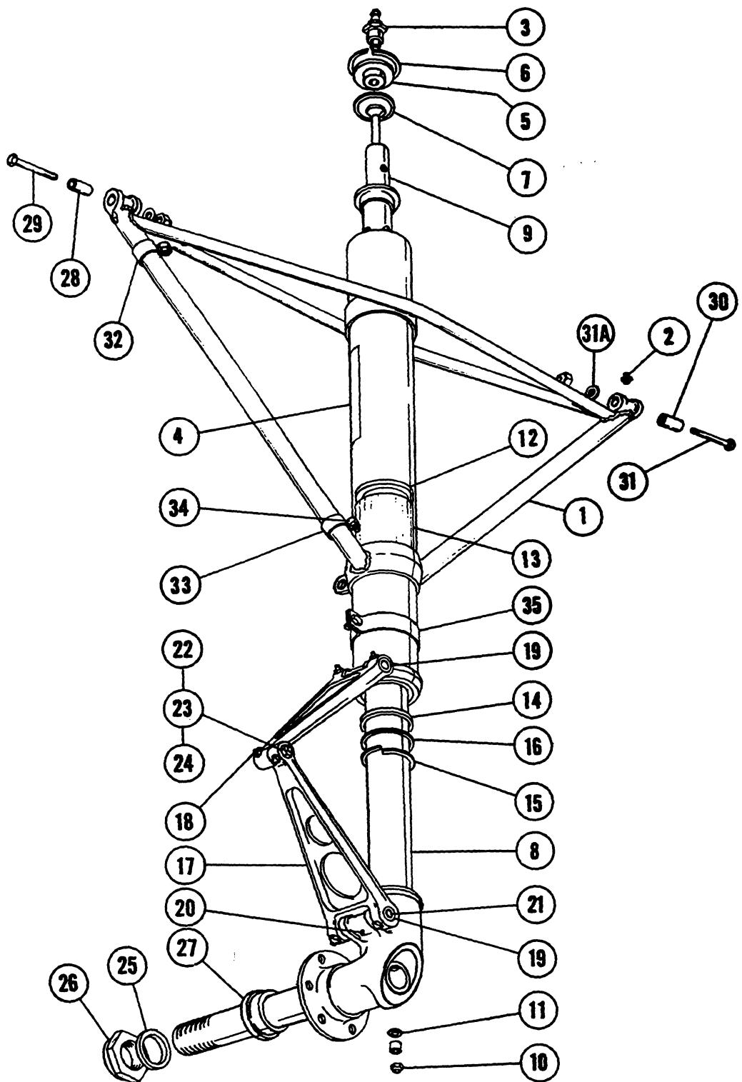
Figure 45. Landing Gear Shock Absorber Assembly (D4099 thru D4865)
