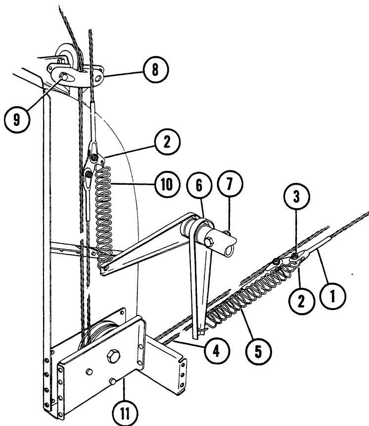
Figure 23. Aileron Bungee Mechanism
