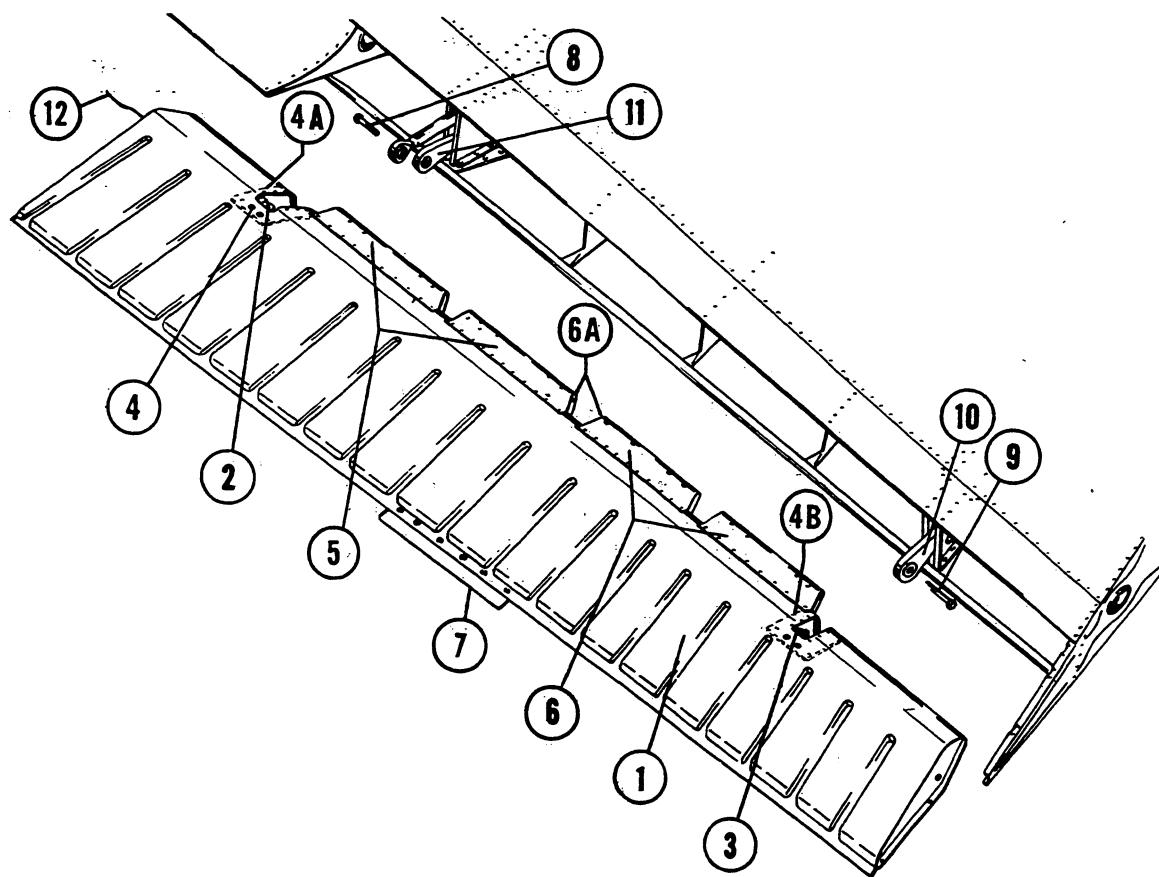
Figure 25. Aileron Assembly
