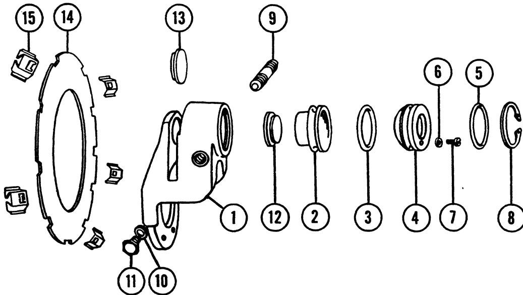
Figure 63. Brake Assembly
