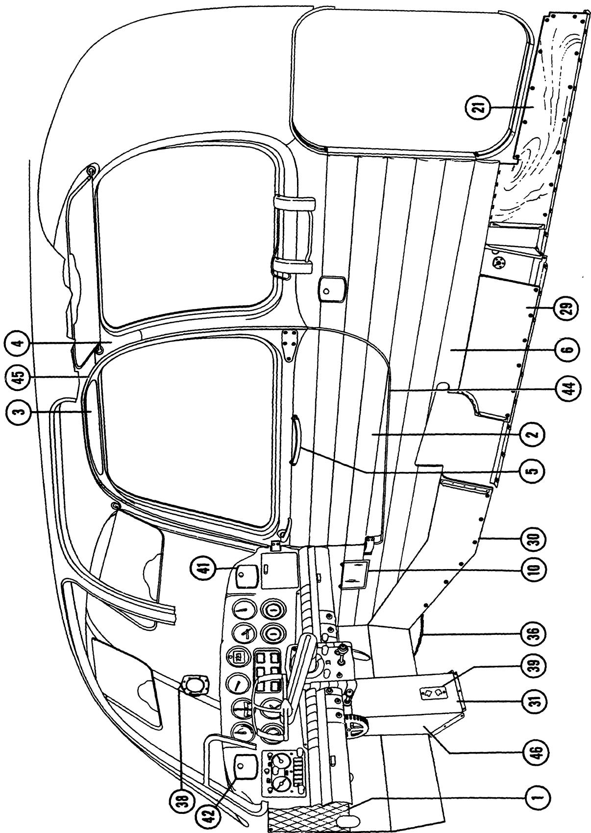
Figure 108. Cabin Furnishings (D2681 thru D4865) (Sheet 1 of 2 Sheets)
