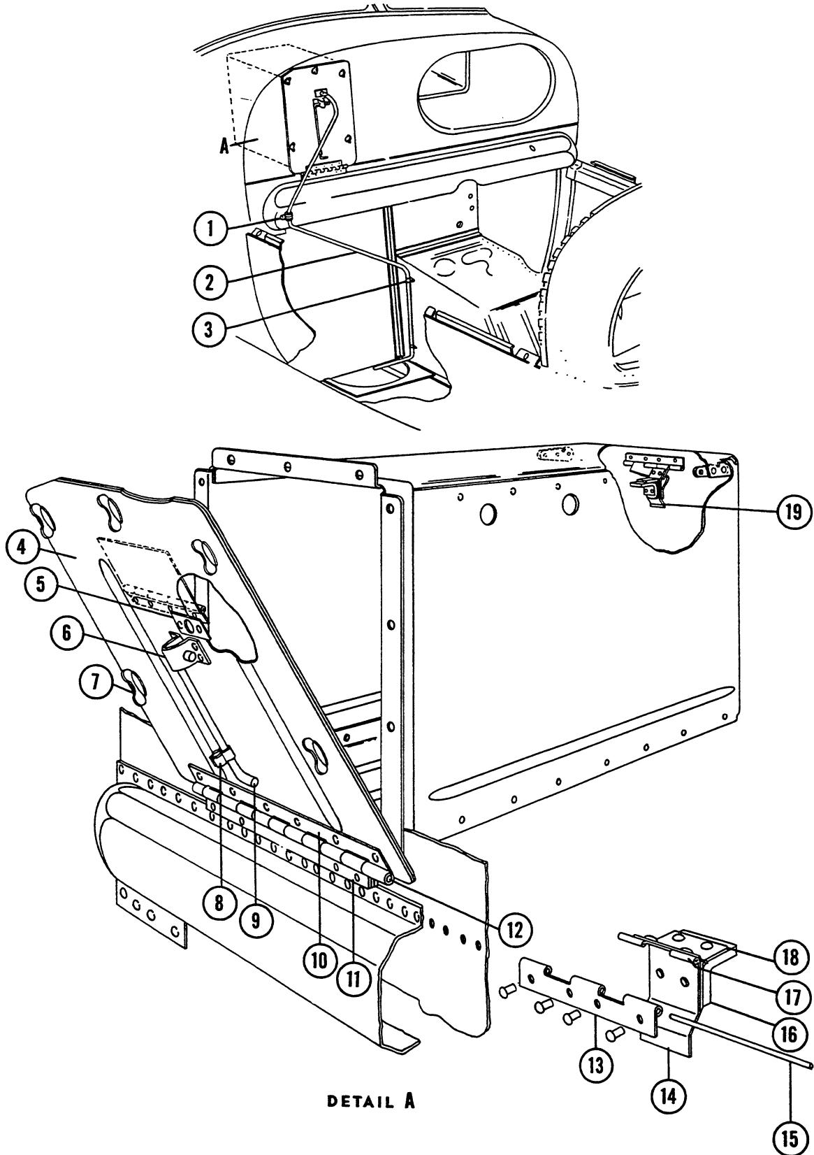
Figure 132. Battery Box Assembly (D1117 thru D1910)
