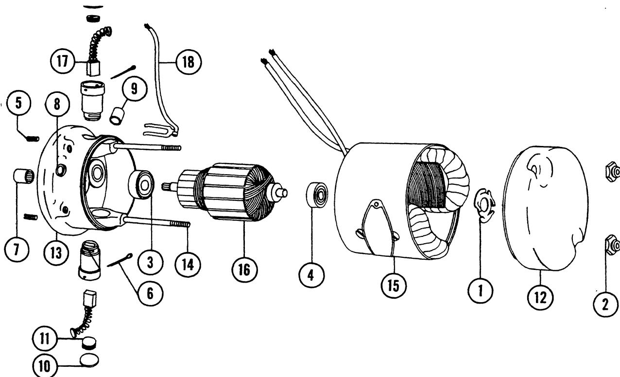
Figure 61. Landing Gear Retract Motor Assembly
