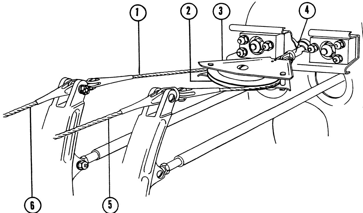
Figure 27. Aft Rudder Control System
