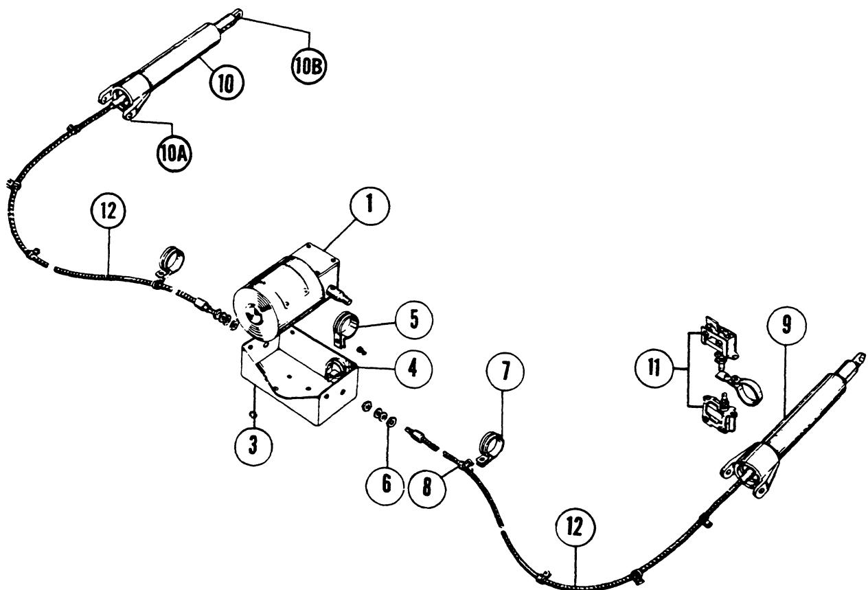
Figure 15. Flap Control Mechanism (D-838 thru D-4865)
