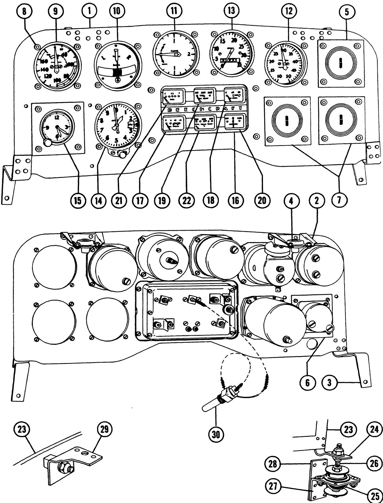
Figure 112. Standard Instrument Panel Assembly (D1 thru D4391)
