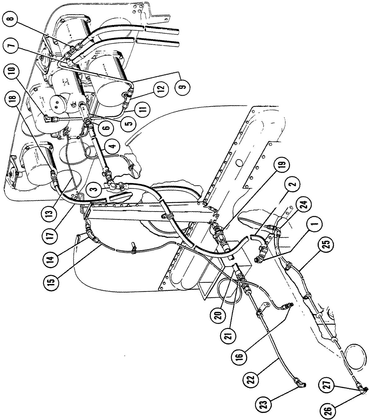
Figure 117. Instrument Plumbing System
