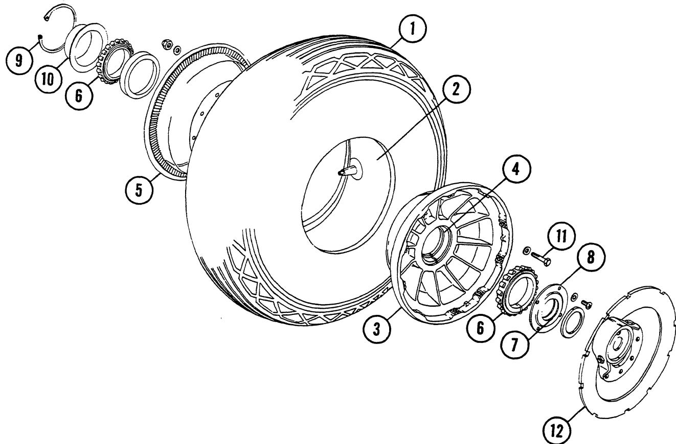
Figure 47. Main Wheel, Tire, Tube And Brake Assembly
