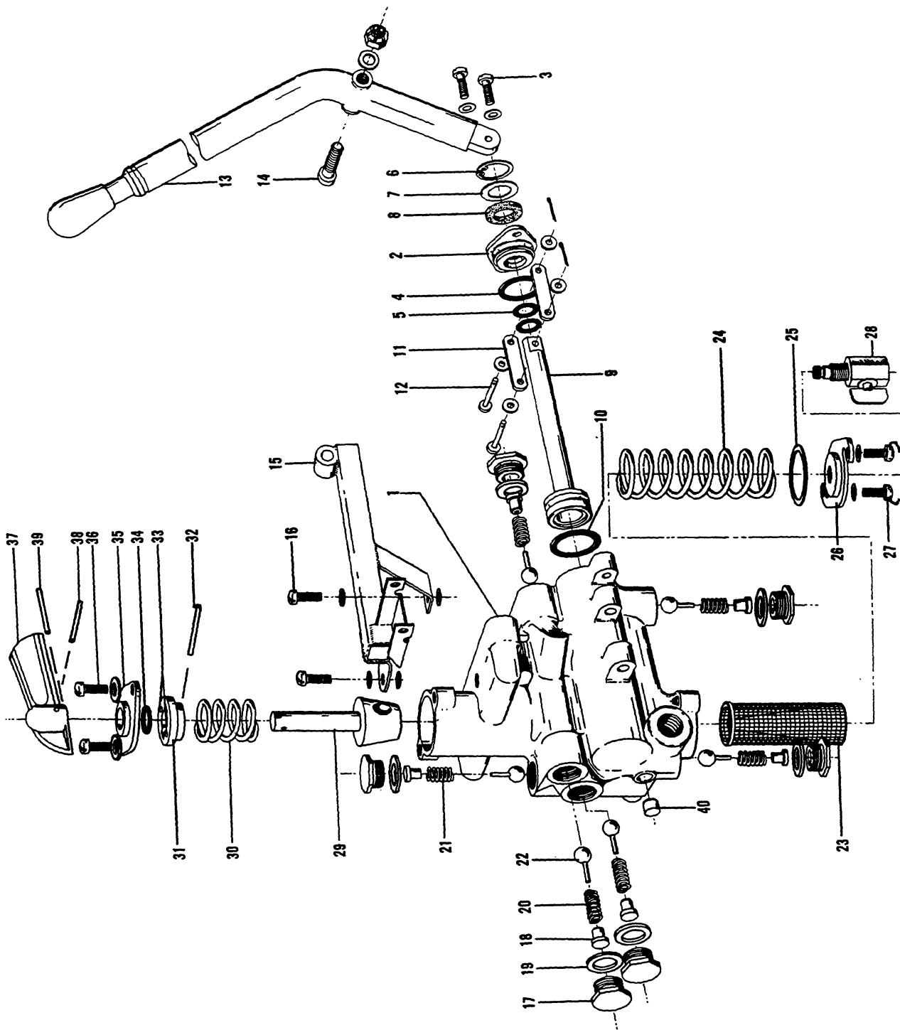
Figure 81. Fuel Unit Assembly (D2901 thru D4865)
