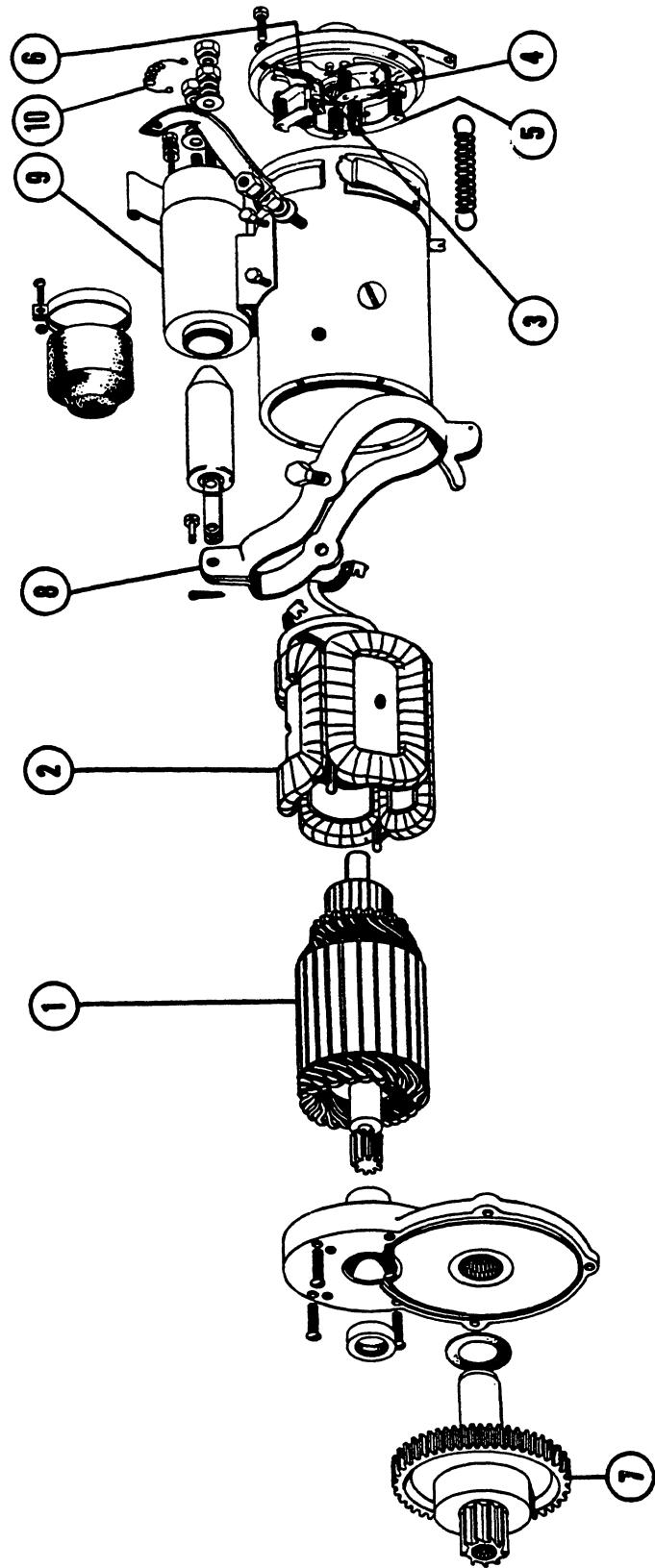
Figure 91. Starter Motor Assembly (D1 thru D1649)
