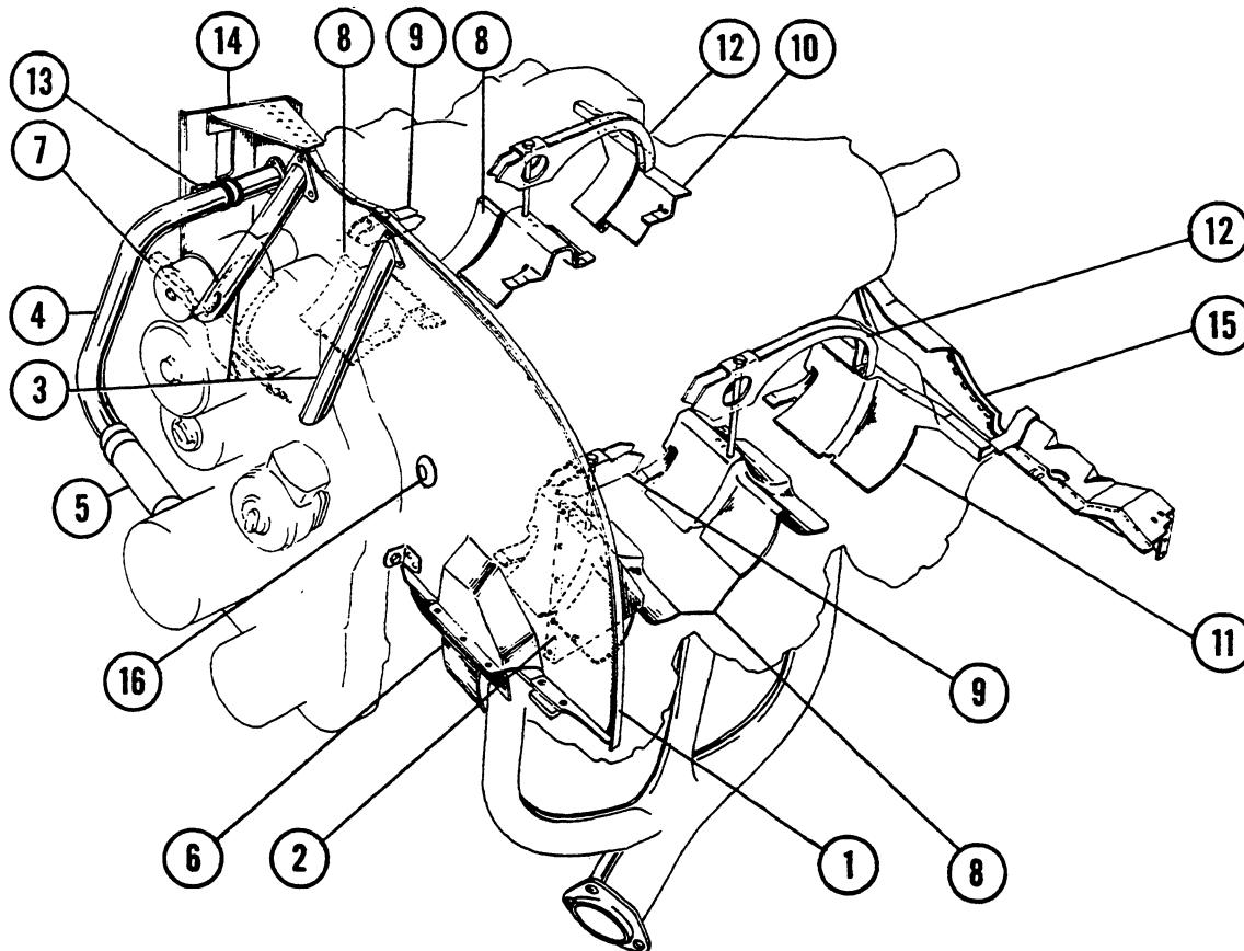
**Figure 74. Engine Baffles**
