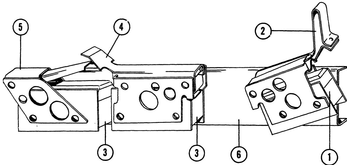
Figure 58. Landing Gear Switch Assembly
