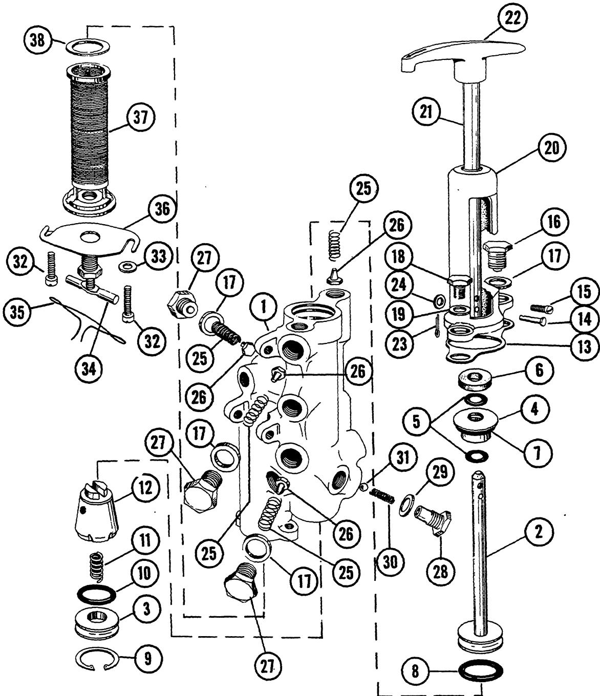
Figure 80. Fuel Unit Assembly (D1 thru D2900)
